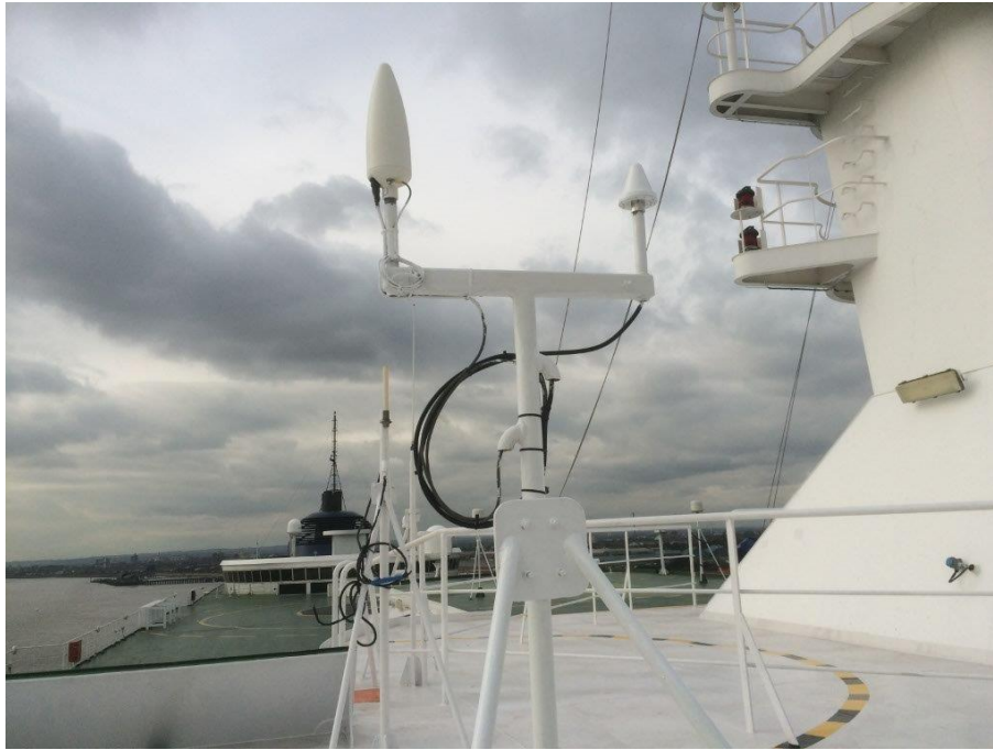
Figure 12 - GPS (right) and combined eLoran/DGPS radiobeacon antenna (left) installed on the Pride of Hull.
