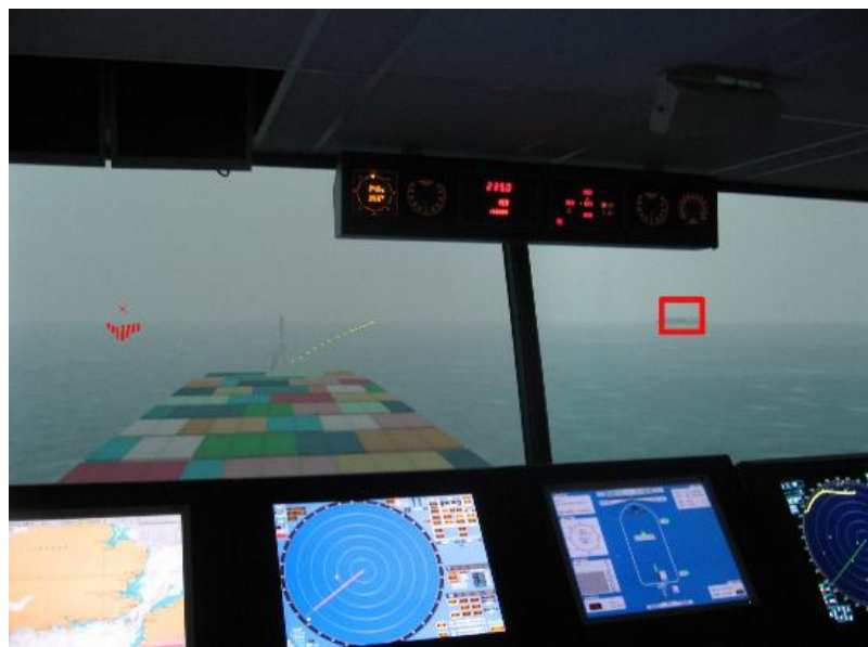
Figure 4 - Display of Suggested Route and a No-Go Area on the HUD.
